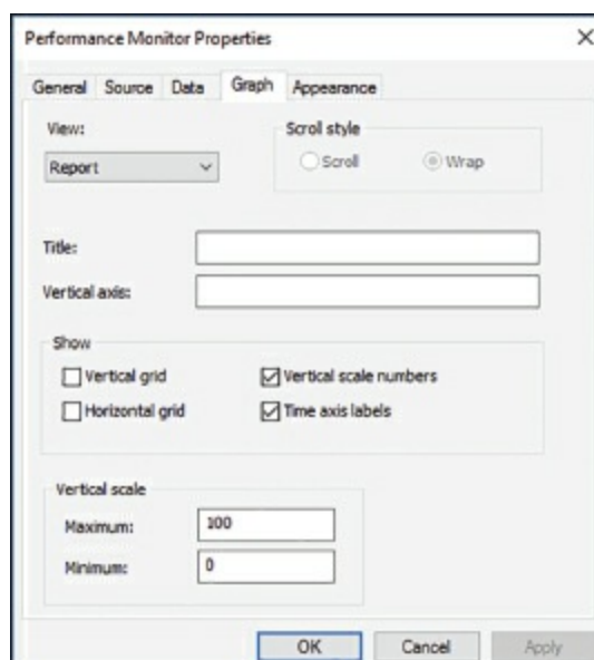
FIGURE 9.8 The Graph tab of the Performance Monitor Properties dialog box
