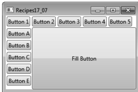
Figure 17-5. Arranging UI elements in a DockPanel
