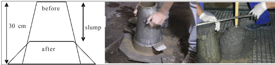
Figure 2. Testing process using the Abrams cone
