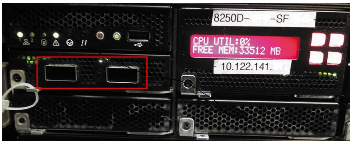
Figure 10-9 Cisco Firepower Appliance Stacking Module
