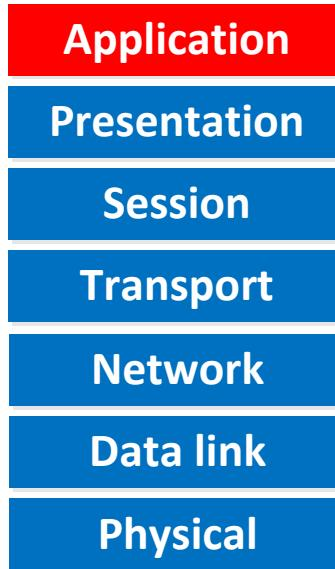
**Top-down** means we start at the top of the OSI model (application layer) and work our way further down to the bottom. The idea is that we will check the application to see if it's working and assume that if a certain layer is working that all the layers below are also working. If you send a ping from one computer to another (ICMP) you can assume that layer 1, 2 and 3 are operational. The downside of this approach is that you need access to the application that you are troubleshooting.
