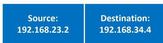
The destination IP address is our webserver and reaching it is no problem. The source IP address is 192.168.23.2 and since we got a response we know that the ISP router knows how to reach the 192.168.23.0 /24 subnet. This makes sense because the 192.168.23.0 /24 subnet is directly connected to the ISP router.
